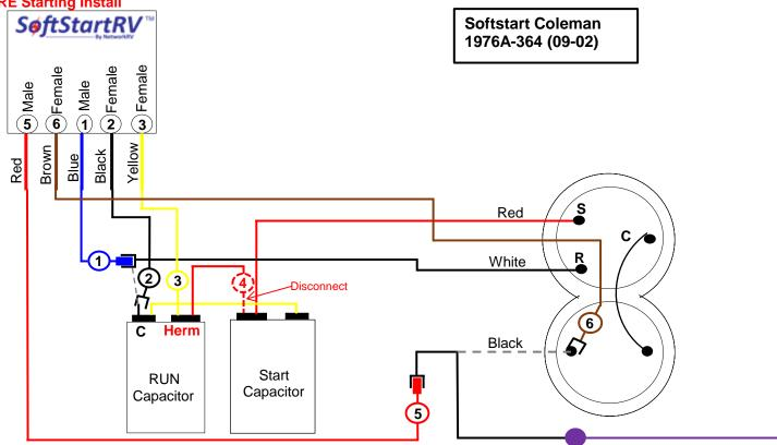
Route Blue, Black and Yellow softastart wires into the ele box, Route Brown and Red to top of compressor, Crimp disconnect as shown in Softstsrt box above Make Sure all disconnects are crimped on tight and are tight when connect to terminals and other disconnects.
