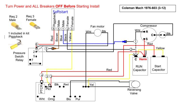
Route ALL Softstart wires into electrical box, Then Crimp Disconnects on wires as shown in Softstart box above
