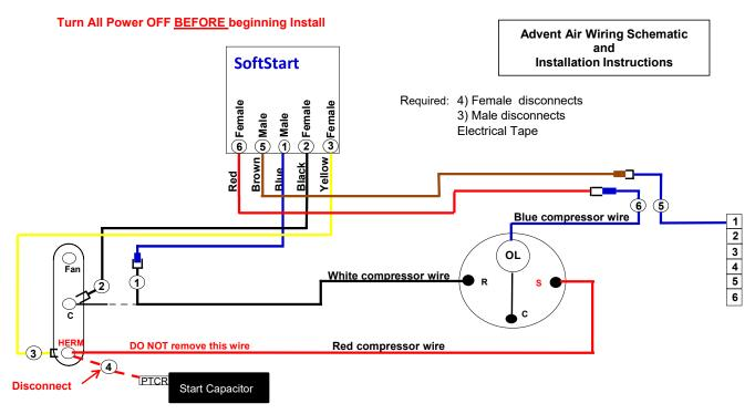
Begin by routing Blue, Black and Yellow Softstart wires into the electrical box. Then Crimp Disconnects on all softstart wire as indicated in Softstart Drawing
